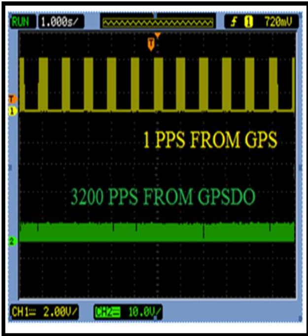
Fig. 6. 1 PPS from GPS and Respective output pulses of GPSDO
